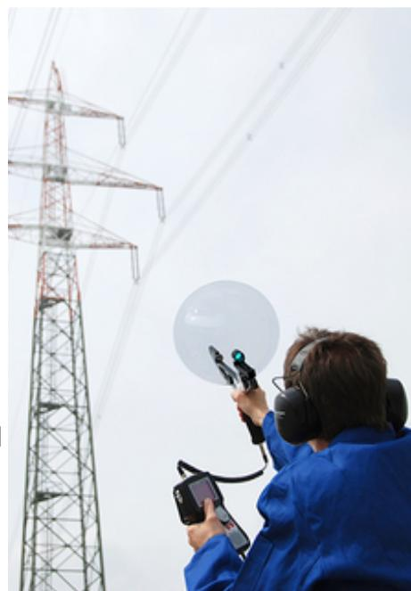
The insensitivity of the SONPAHONE to interfering noises in the scope of audible sound offers optimum prerequisites for application in noisy industrial environments. Thanks to the multi-functionality of the SONAPHONE devices and the coordinated accessories, costs are saved in many areas because searching for faults is easier and can proceed more quickly.
