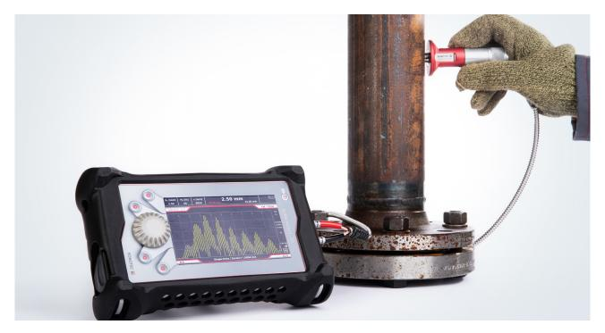
High Temperature Thickness Measurement with SONOWALL 70 and ultrasonic probe SONOSCAN TS5H
