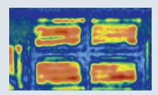
Test method: Transmission Type of defects: air pockets, electrolyte distribution
