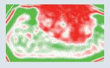
**Test method:** Transmission **Type of defects:** delamination and density fluctuations before and after the sintering process
