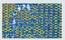
Test method: Transmission Types of defects: impact damage and delaminated top layer Probe: CFC230\_D25\_P65
