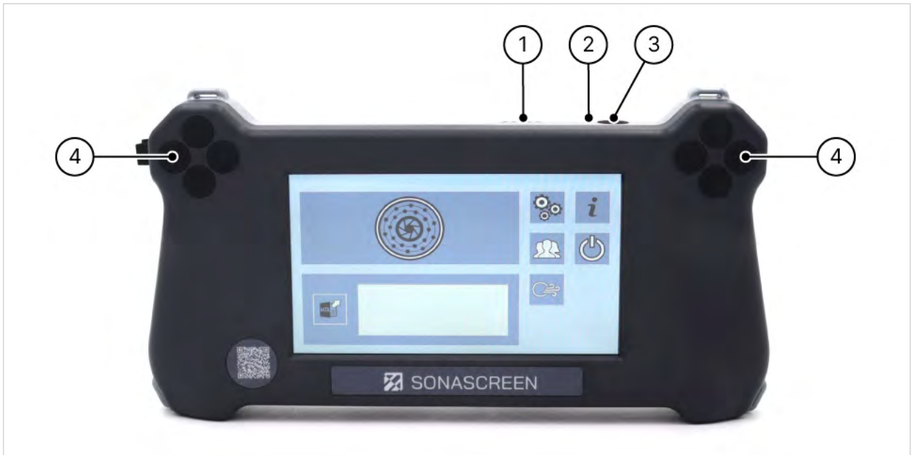
Figure 2: Operating side with status display and device buttons
