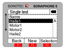
By pressing function key "F2" you can create a new Single test, by turning the rotary knob you can edit the current Single test, and you are able to activate the selected Single test by pressing "F3".
