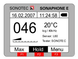
Press the rotary knob to store the currently <u>displayed value</u>, in other words the "Hold" value, in the individual test that is active.
