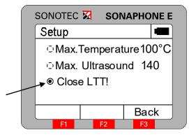
All test values, which have been recorded until this point, are kept and displayed in the overview of the Long-time tests, which are stored in the device.
