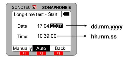
When this menu is opened, the start of the Long-time test is set to "Auto". The SONAPHONE E will thus start the Long-time test automatically at the time that has been set. If the time entered is earlier than the present time, the test is started immediately.
