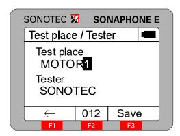
The character to be edited is selected by pressing the rotary knob and set by turning it. To edit the last character again press the Button "F1". The character sets ( $ABC \rightarrow abc \rightarrow 0.12 \rightarrow .;<$ ) are switched over by pressing the "F2" key. Press "F3" to store both the tester's name and the test site for the corresponding Single test.
