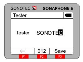
The character to be edited is selected by pressing the rotary knob and set by turning it. Press "F3" to store the tester's name in the device.
