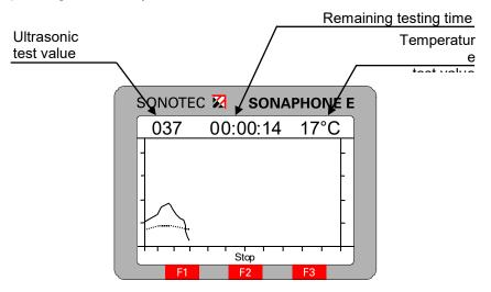
The ultrasonic test values are represented by a solid line, and the temperature values by a dotted line. The remaining time of the test is shown at the top center of the screen. The Long-time test can be cancelled at any time by pressing function key F2. The values recorded up to that time are stored and the entry for the duration of the test is updated.
