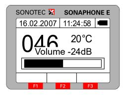
Turning the rotary knob clockwise increases the volume and turning it anti-clockwise decreases the volume.
