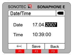
The element to be edited is selected by pressing the rotary knob, and set by turning it. To edit the last element again press the function key F1. Pressing function key F2 stores the time. Pressing function key F3 deletes the settings and returns the unit to the previous menu.
