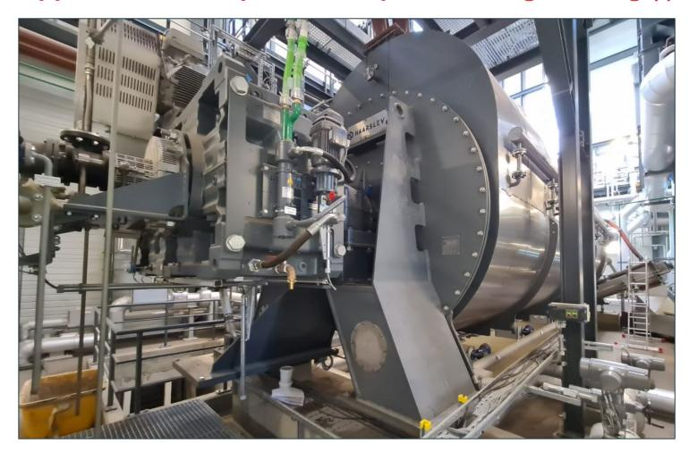
Slow speed dryer, payload 26 tons, 7.4 rev/min
