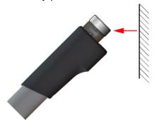
3. Carefully push the protective pad sideways on the magnetic waveguide.
