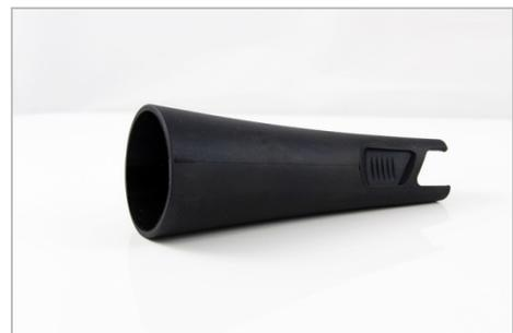
If the systems and system components being tested are large distances apart, the large acoustic horn should be used to narrow down the search area. The funnel pools the ultrasonic signals over large distances, allowing for verification with the SONAPHONE. Areas where ultrasonic signals can be verified in this way can then undergo precise location using the precise locator BS10-1.
