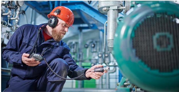
→ Detect bearing damage early and optimize bearing lubrication
