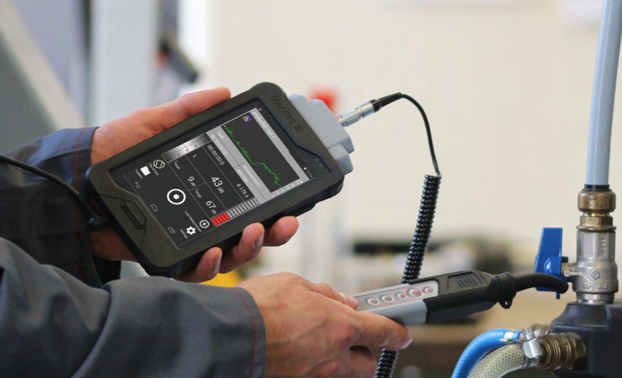
SONAPHONE Digital ultrasonic testing device for maintenance 4.0
