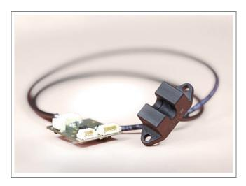
The **BLD02** is a **non-invasive**, **optical sensor** with remote electronics (probe and PCB) developed to detect smallest amounts of blood in a clear fluid from the outside through transparent plastic tubing.
